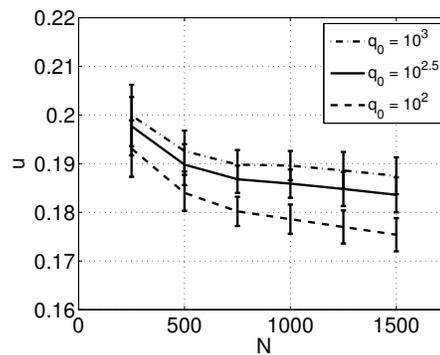
Fig. 1. The dimensionless function  $u$  for four directions and  $\nu = 10$  as a function of  $N$  for different values of  $q_0$ .
