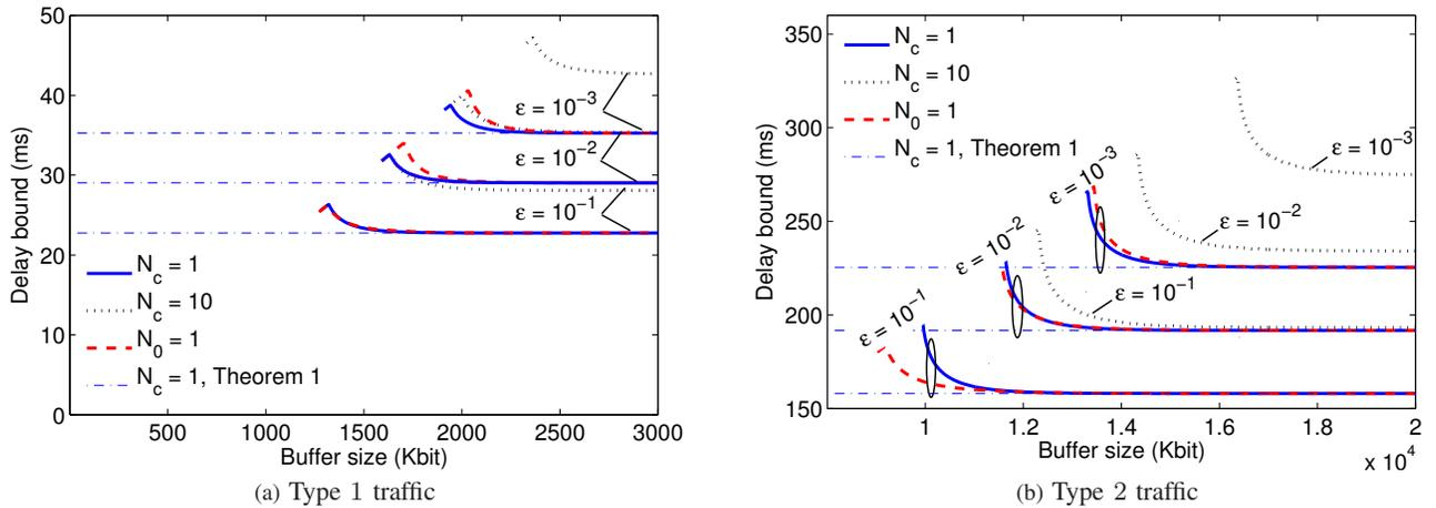
Fig. 5: The impact of considering finite buffers on per-flow delay computations;  $\varepsilon = 10^{-1}, 10^{-2}, 10^{-3}$ ,  $N = 300$ ,  $N_0 + N_c = N$ ,  $A_0$  is either very tiny (when  $N_0 = 1$ ) or very large (when  $N_c = 1, 10$ ), relative to the aggregate  $A_0 + A_c$ , utilization = 90%, and the source types from Table I (Type 1 (less bursty) in (a) and Type 2 (more bursty) in (b)); for  $N_c = 1$ , the infinite buffer approximation result (with Theorem 1) is also shown.
