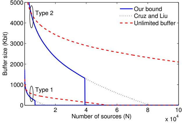
Fig. 3: Comparison of three aggregate loss probability bounds. We fix the loss probability  $P^{loss} = 0.1$ , the utilization = 90%, and plot the required buffer size as a function of the total number  $N$  of sources, for the two types from Table I.
