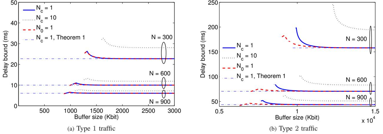
Fig. 4: The impact of considering finite buffers on per-flow delay computations;  $\varepsilon = 0.1$ ,  $N = 300, 600, 900$  with  $N_0 + N_c = N$ ,  $A_0$  is either very tiny (when  $N_0 = 1$ ) or very large (when  $N_c = 1, 10$ ), relative to the aggregate  $A_0 + A_c$ , utilization = 90%, and the source types from Table I (Type 1 (less bursty) in (a) and Type 2 (more bursty) in (b)); for  $N_c = 1$ , the infinite buffer approximation result (with Theorem 1) is also shown.
