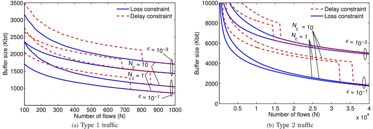
Fig. 6: Comparison of buffer size provisioning methods based on through flow loss constraint (i.e.,  $P_{K,0}^{loss} = \varepsilon$ ) and delay constraint as a function of total number of flows  $N = N_0 + N_c$ , utilization=90%, and the source types from Table I (Type 1 (less bursty) in (a) and Type 2 (more bursty) in (b))
